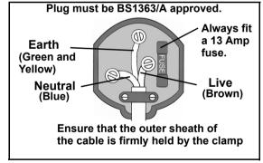
connected to the terminal which is marked E or  $\pm$  or coloured green.
